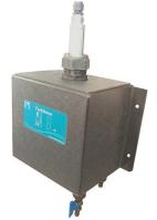
TurbSense turbidity sensor in flow cell
