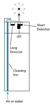
concentrations of solids. The SoliSense<sup>®</sup> uses Pi's novel measurement technique that automatically takes readings at four different light levels and uses the gradient between the four readings to produce the sensor output. This configuration allows accurate and reliable measurements of suspended solids concentrations and turbidity to be made.
